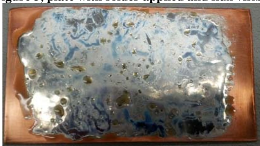
Figure 3, plate with solder applied and flux visible
