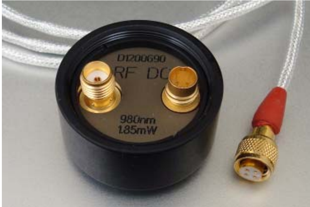
Figure 4, rear view of laser diode head showing bias and RF modulation inputs. The 1.85mW power is residual from a previous laser diode, and is not applicable to this design.
