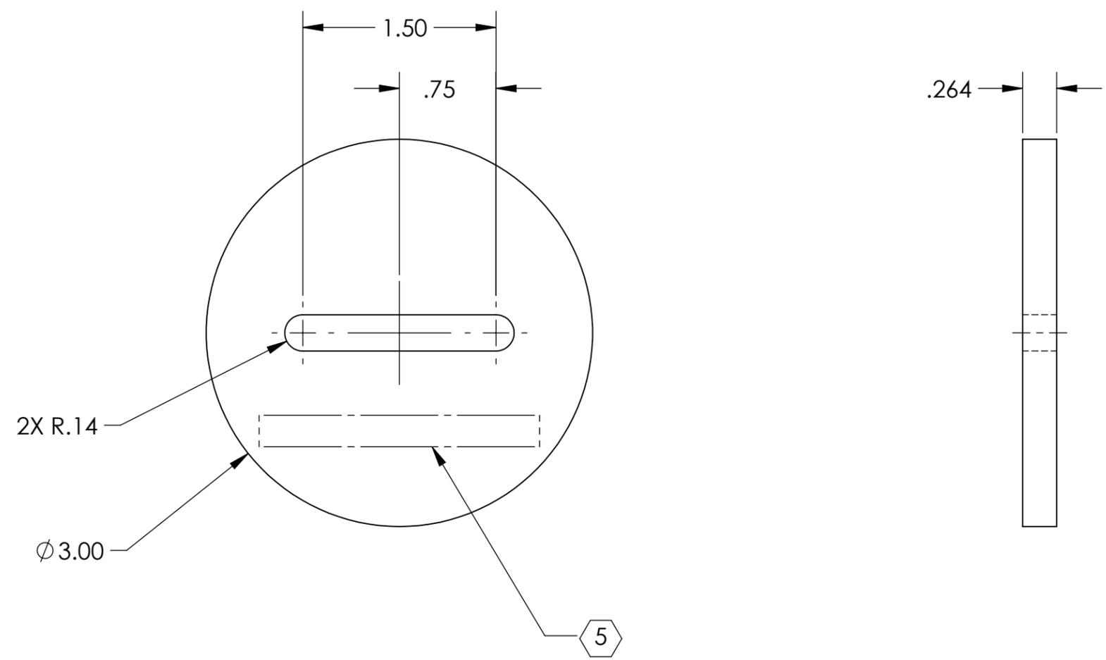
D1201230\_AdlIGO\_slc Half Pound BalanceWeight, PART PDM REV: X-001, DRAWING PDM REV:
