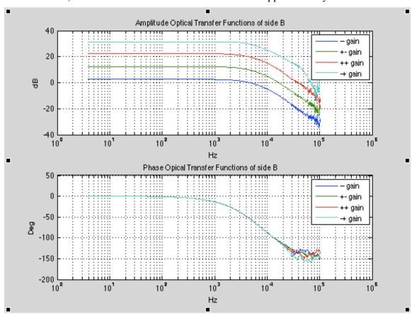
We can compare the optical transfer function with the electrical transfer function. Below is a plot of this comparison for board side B at the highest gain. They are pretty similar.
