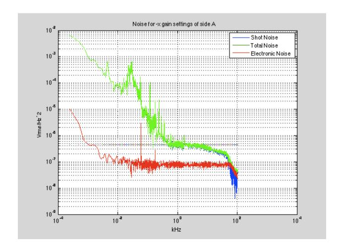
Again, these noise measurements were repeated using a long cable (100ft). Below is a graph of the electrical noise, and the shot noise of side A at the lowest gain setting for both the long and short cable. Evidently, there is not much of a difference between the two cables in terms of noise.
