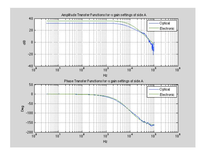
We repeated the measurements for the optical transfer function using a long cable (100ft). The results were consistent. Below is a plot comparing the two transfer functions for board side A at the highest gain.
