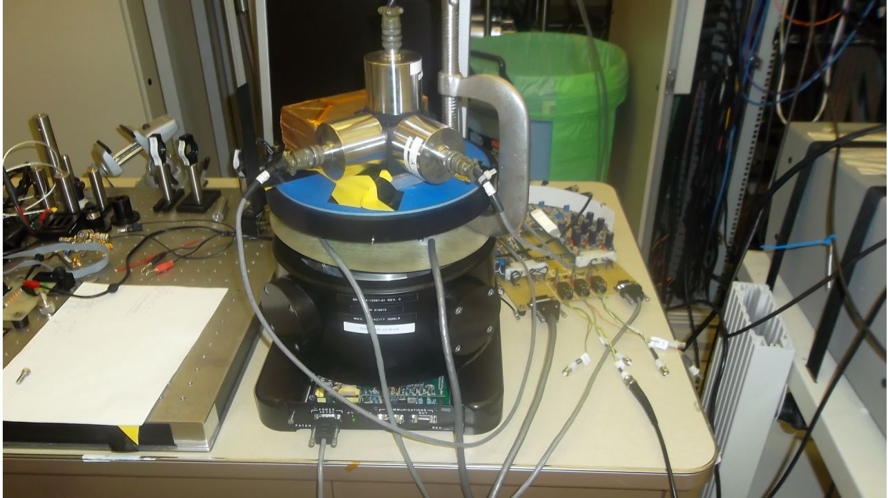
Figure 1: The STACIS unit I am working with. The cylinders on top are the accelerometers; the internal geophones are not visible. The x and y PZTs are the horizontal cylinders protruding midway up the STACIS, and to the right is the extension board that allows access to some of the electronics.
