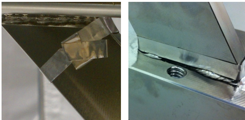
Figure 24. a) and b) Covering notches with Al strips
