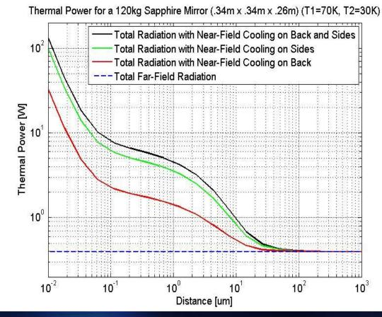
Conduction through the fibers: 4.4x10<sup>-6</sup> W/K (<< far field radiation)
