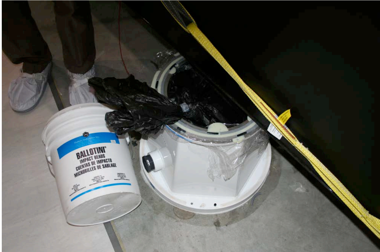
Figure 1 aLIGO PSL table leg test after lifting table off of legs. The leg is grouted to the LVEA floor using Hydrostone. The table “floats” on sections of Viton o-rings until an annular bead of epoxy hardens, thus equally loading the six legs and making a hard vertical connection.
