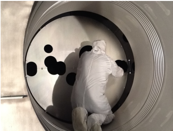
Mode Cleaner Tube baffles for recycling cavities
