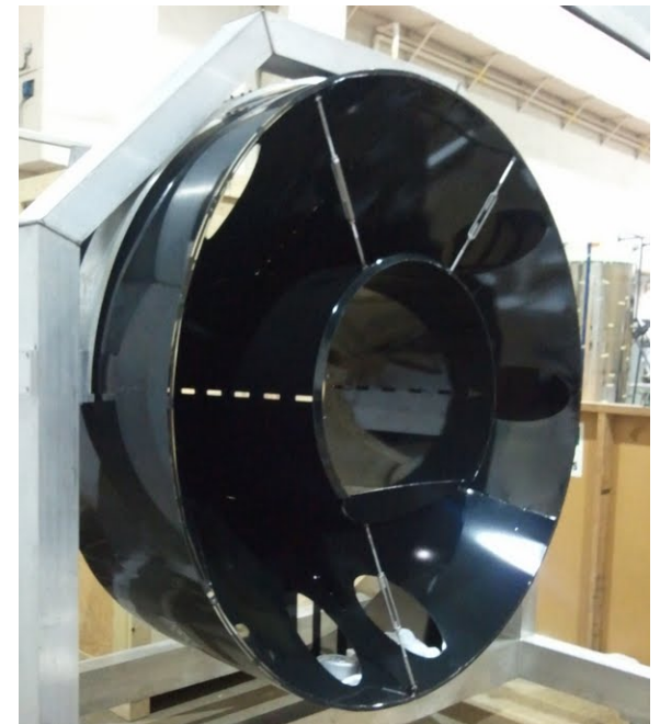
Assembly and vibration testing of prototype, suspended Manifold/ Cryopump Baffle at Caltech
