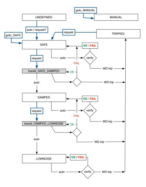
example state diagram for a triple suspension is included below.
