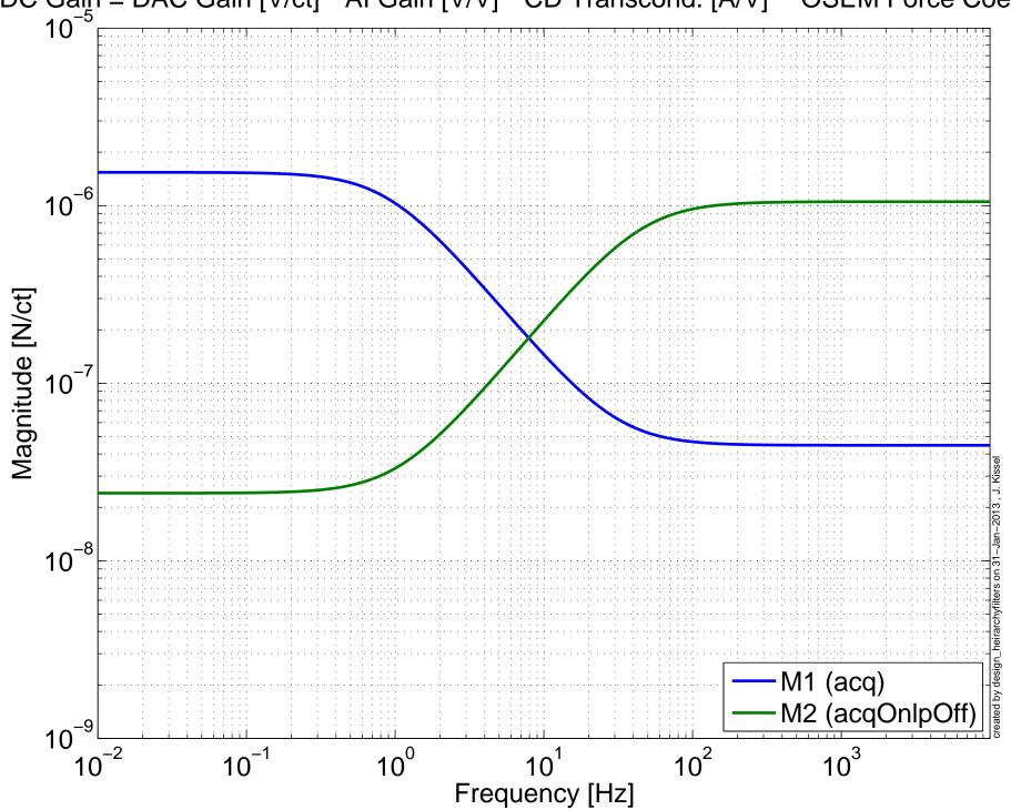
BSFM Transfer Function, L to L Response at Optic to Drive at Each Stage
