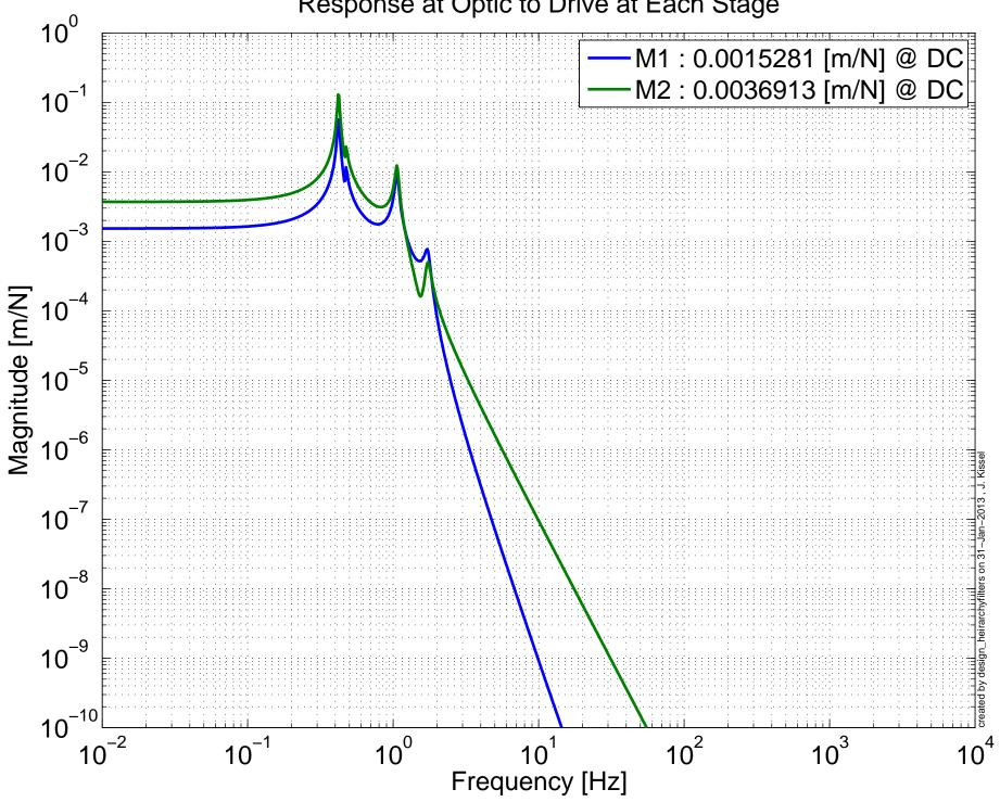
BSFM Transfer Function, P to P Response at Optic to Drive at Each Stage
