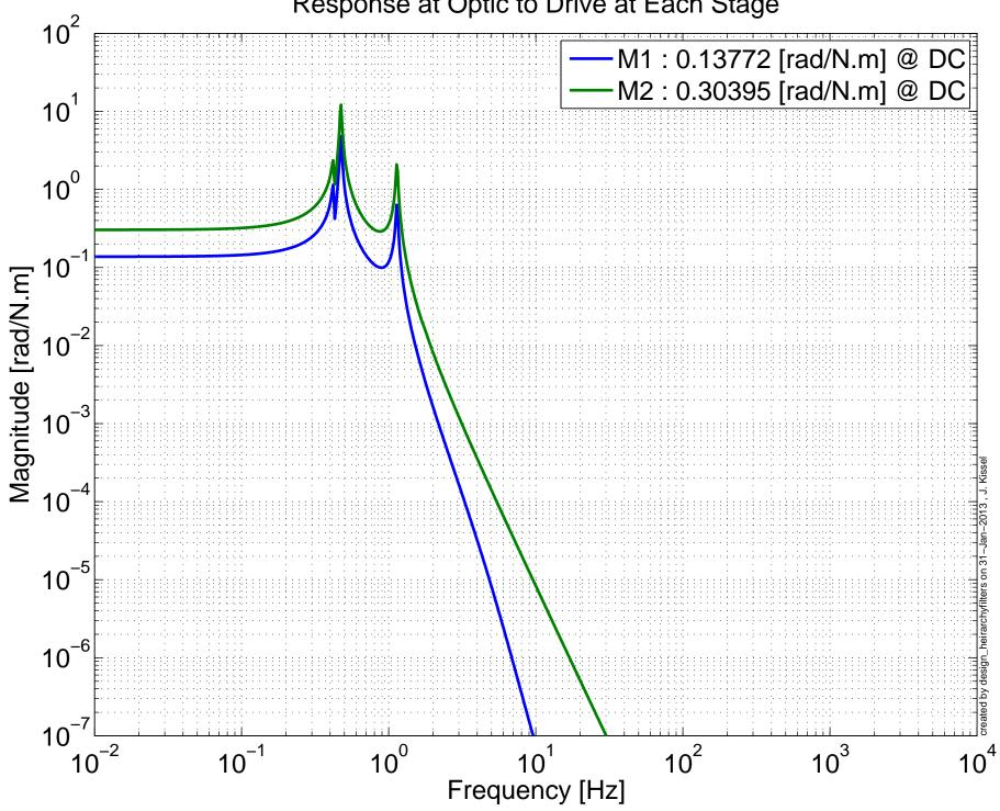
BSFM Transfer Function, Y to Y Response at Optic to Drive at Each Stage
