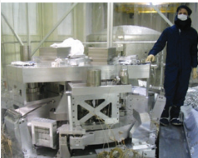
c) The new vibration isolation system includes of a hydraulic pre-isolator and an active internal isolator.
