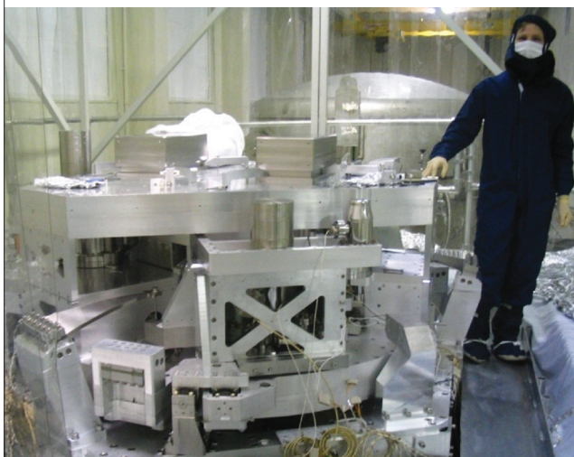
c) The new vibration isolation system includes of a hydraulic pre-isolator and an active internal isolator.
