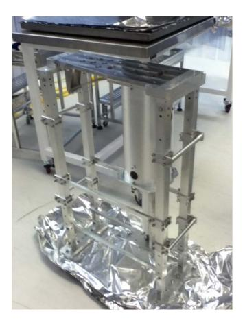
6 - Replace and fasten the **Upper Clamp** with the saved hardware.
