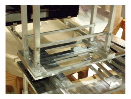
6.2.3 The two people inside the chamber will adjust the Table, Secondary, Suspension" (D1101962) so that it is directly below the Stage 0 position where the ACB suspension will be attached.
