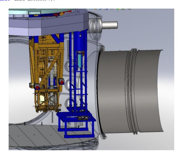
8.4.13 Slowly turn the Jacks and raise the lifting table upwards until the Installation Stand touches the Suspension Assembly.
