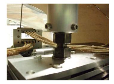
3.2.10 Slowly crank the lifting table downwards until the lifting table is approximately one inch below the bottom of the ACB box.
