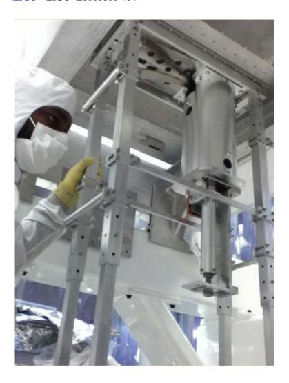
3.1.11 Remove Side Beam from Installation Stand from each side one at a time, clamping that side with Dog Clamps before removing the other side. Remove parts and set aside.
