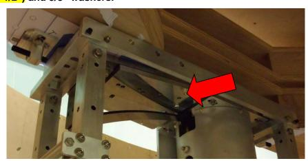
6.2.15 Remove four 1/4-20 SHCS and "SIDE BEAM" (D1102026) from Installation Stand on the side closest to the chamber wall. Remove from vacuum system.
