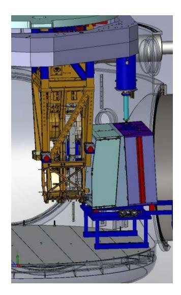
8.3.8 Detach the four captive screws that attach the Top Hinge Plate on Suspension Assembly to Bottom Hinge Plate on Baffle Box Assembly.
