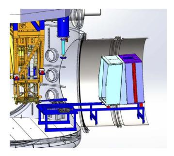
6.3.5 The Slide Assembly feet have Teflon pads that allow for an easy slide down the rail. There are blocks attached to the end of the rails to prevent travel past the Table end. Slide the Baffle Box toward the QUAD until it is positioned directly above the Wedge Lift, Baffle, Suspension Table" (D1101952, stopping at the approximate location needed to raise and mate the Baffle Box Assembly with the Suspension Assembly.
