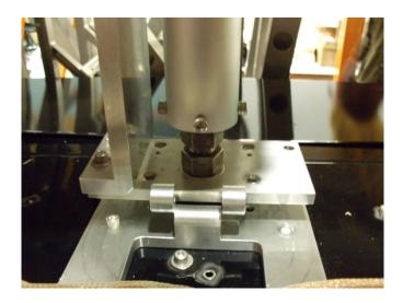
3.2.8 Attach Baffle Box Assembly to Suspension Assembly with Shoulder Screw (D1101293), three #10 Flat Washers, and one #10-24 Silver Plated Nut
