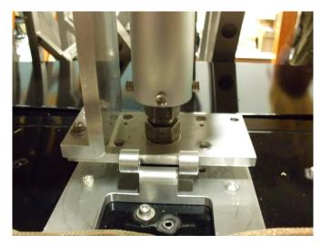
6.3.7 Attach Baffle Box Assembly to Suspension Assembly with one #10-24 Shoulder Screw (D1101293), three #10 Flat Washers, and one #10-24 Silver Plated Nut
