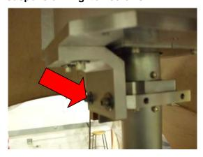
6.5.6 Verify balance of baffle. Shift balance weights as needed axially and laterally until the "SLC Baffle Tube Up Assembly" (D1002582) is evenly spaced inside "SLC Earthquake Stop Ring" (D1001120) circumference.
