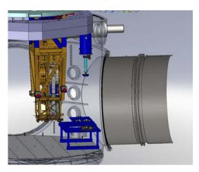
6.2.22 Remove the twelve 1/4-20 SHCS attaching the Secondary Table to the Suspension Lift Assembly. Place SHCS on aluminum foil container in bottom of spool for use in next step. Carefully remove the Secondary Table from vacuum system.
