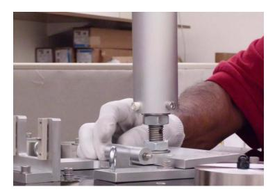
3.2.9 Attach four captive 1/4-20 SHCS in the Top Hinge Plate on Suspension Assembly to Bottom Hinge Plate on Baffle Box Assembly.
