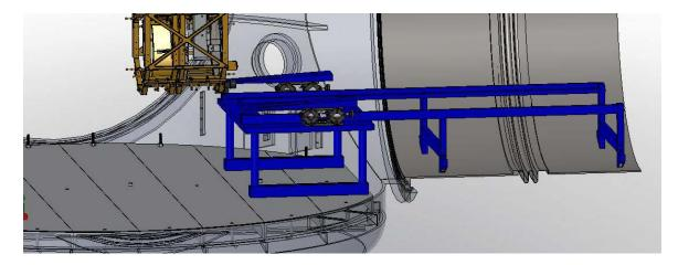
6.1.5 Attach the "Rail, ACB Assembly" (D1101724) to the "Suspension Lift Assembly" (D1101953) using two SHCS (1/4-20 x .62").
