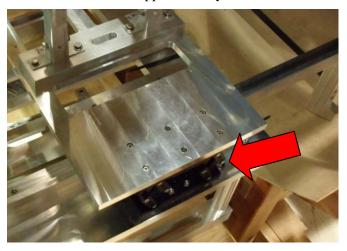
6.2.12 The two people on each side of the Table uniformly raise the Jacks to lift the Installation Stand and align Interface Mounting Plate to STAGE-0 mounting locations. Continue until top of Interface Mounting Plate touches STAGE-0.
