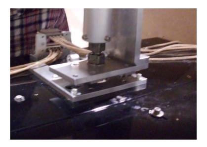
8.3.9 Remove the Shoulder Screw, #10 Flat Washers, and #10-24 Silver Plated Nut that attach the Baffle Box Assembly to the Suspension Assembly.
