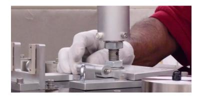
6.3.8 Attach four captive SHCS in Top Hinge Plate on Suspension Assembly to Bottom Hinge Plate on Baffle Box Assembly.
