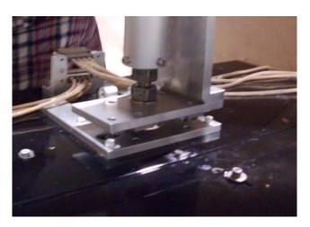
6.3.6 The two people on each side of the Table uniformly raise the Jacks to lift Baffle Box Assembly and align to top hinge plate at bottom of Suspension Assembly. Adjust Baffle Box position as needed for alignment. Continue lifting until hinge plates touch.
