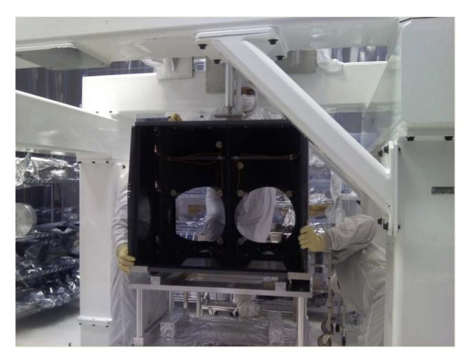
3.2.7 Crank Lifting Table (D1002192) upwards to lift Baffle Box Assembly and align to Top Hinge Plate at bottom of Suspension Assembly. Adjust Baffle Box position by moving the cranked lower lifting table as needed for alignment. Continue lift until plates touch.
