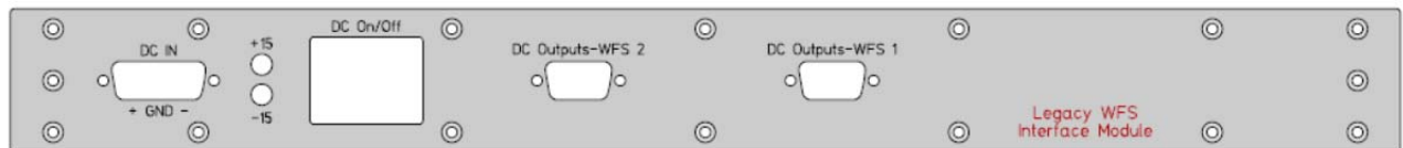
Figure 2: ISC 2 Channel, Legacy WFS Interface, Rear Panel
