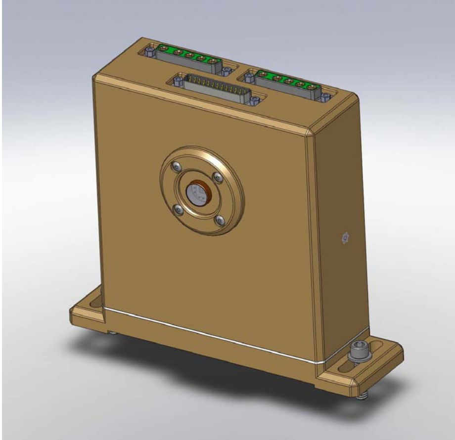
Figure 12. In-air package for the WFS. Photodiode center is at 4 inch height from mounting surface. There are two D-sub, 5-way coax connectors, one for each detection frequency. Each such connector contains the RF outputs for each of the quad segments. One of the D-sub also contains the test input (the remaining coax contact is not used). The box is approximately 6" high, 5-3/8" wide, and 2" deep (not including protrusions).
