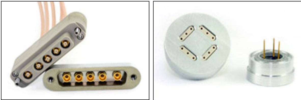
Figure 10. Photodiode feedthrus for the in-vacuum RF detectors. Left: quad photodiode feedthru; photo shows the side the diode plugs into. Right: single element feedthru; photo shows the side that mates to the circuit board. The aluminum holders are laser-welded into an aluminum box that contains the circuit board.
