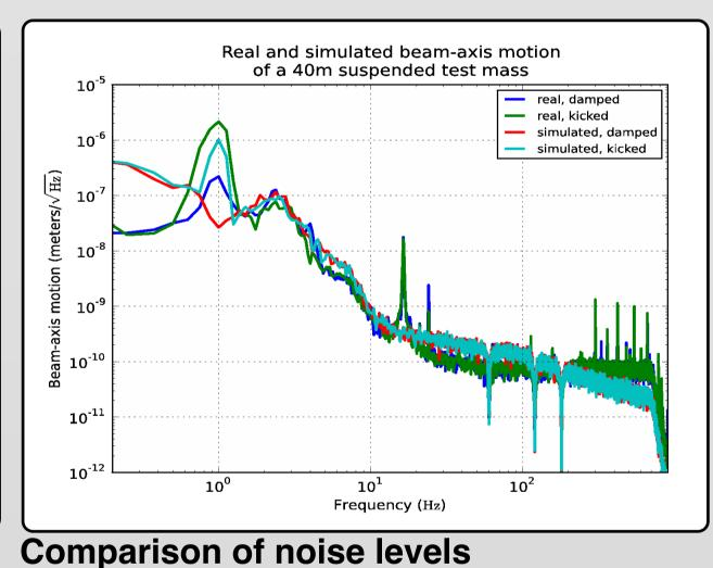
between the simulated and real suspensions
