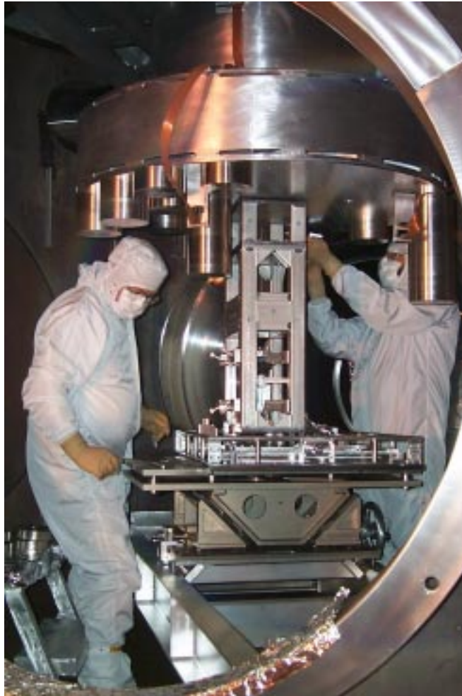
FIGURE 2. The First Folding Mirror Being Installed into BSC Chamber (BSC) #8 in the Y-arm at Hanford, Washington.
