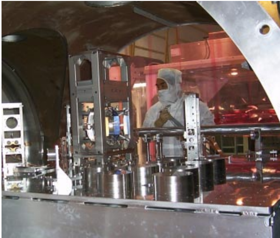
FIGURE 3. MMT3 Optic Installed into HAM Chamber #7 at Hanford, Washington.
