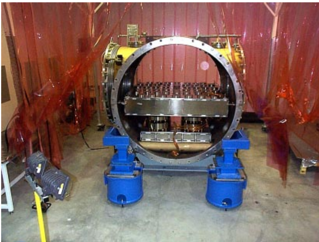
FIGURE 9. Horizontal Access Module (HAM) First Article Seismic Isolation System
