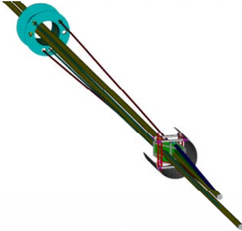
FIGURE 8. Perspective View of the Beams. The pointing beams are shown entering and exiting from viewports mounted in a beam reducing manifold.
