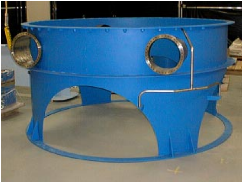
FIGURE 6. Mock-up of the Beam Splitter Chamber (BSC) for First Article Fit Check
