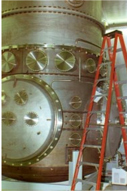
FIGURE 3. Production Beam Splitter Chamber after Cleaning.
