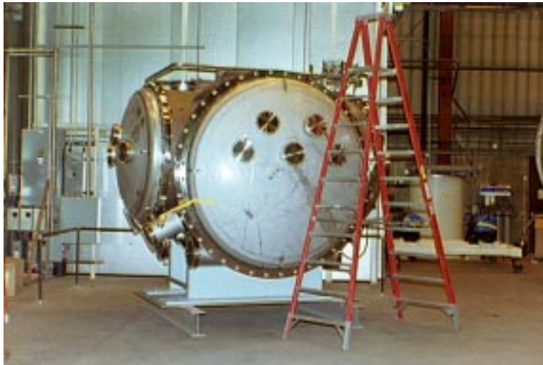
FIGURE 4. Horizontal Access Module Ready for Vacuum Bake and Test.
