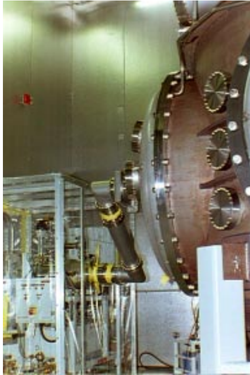
FIGURE 5. Initial Leak Check of Beam Splitter Chamber.
