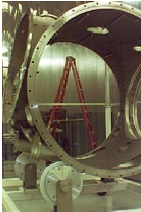
FIGURE 5. Horizontal Access Module Chamber
