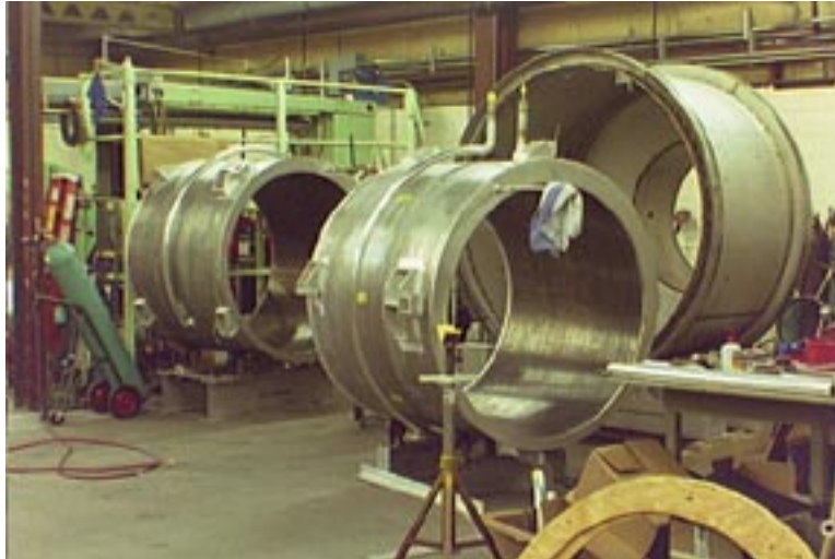
FIGURE 8. 80K Pump Reservoirs
