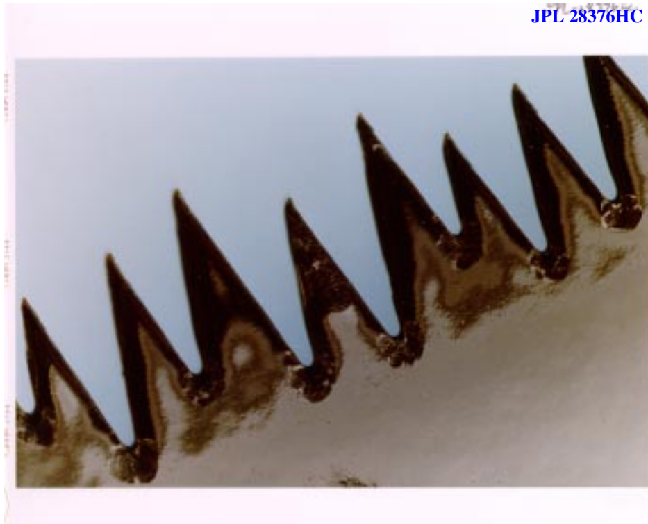
FIGURE 11. Areas of Glass Shedding near Baffle Serrations
