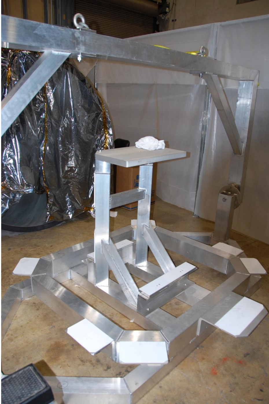
Figure 1: Manifold/cryopump Baffle Assembly and Transport Apparatus
