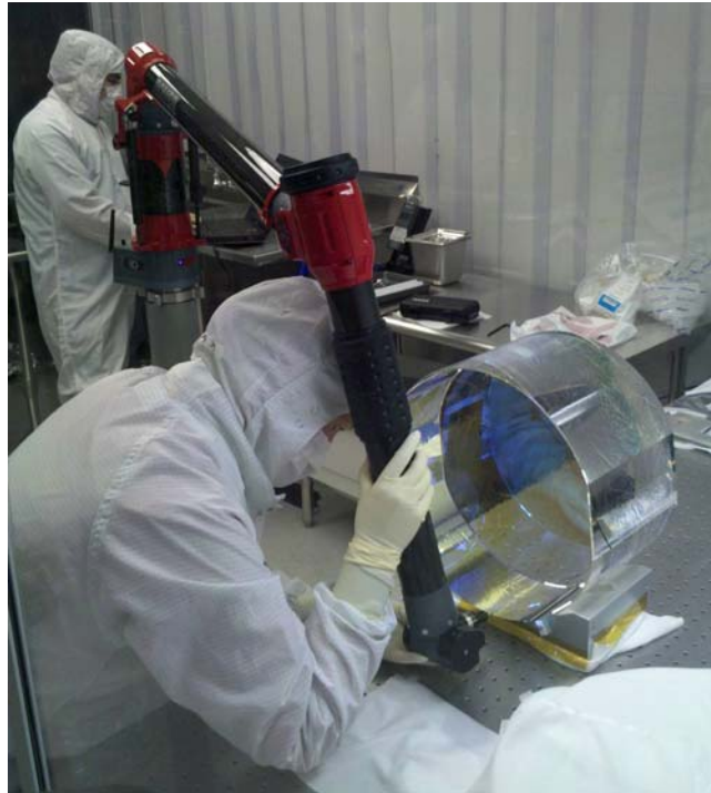
Figure 4.2 Using the Romer arm to measure the width of TM ETM02
