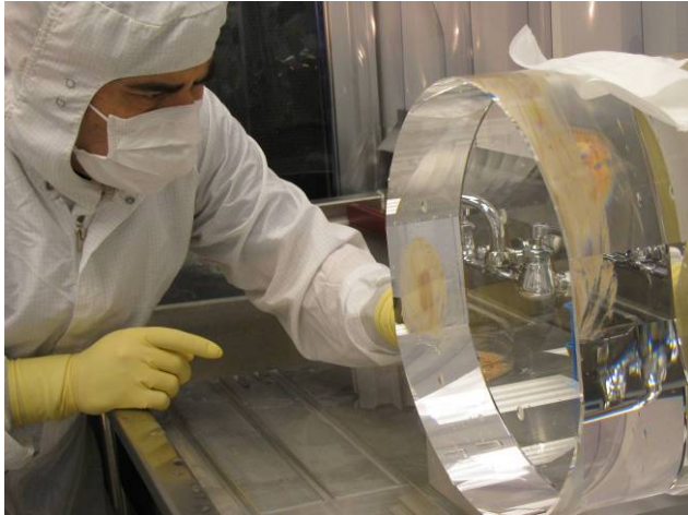
a) Cleaning the bonding surface with cerium oxide
