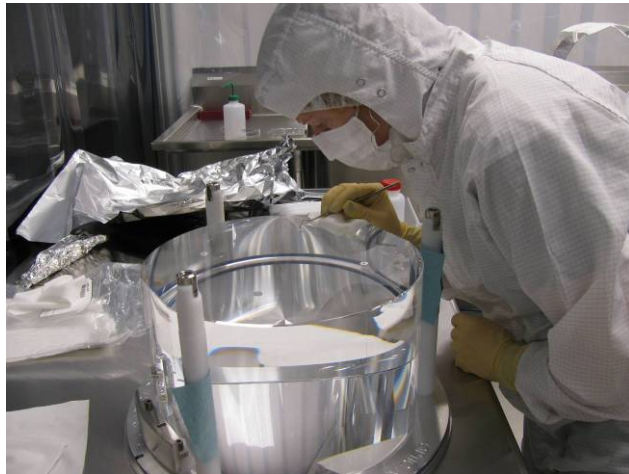
a) Betsy gluing a steel ring onto a mount disc on PM ITM04
