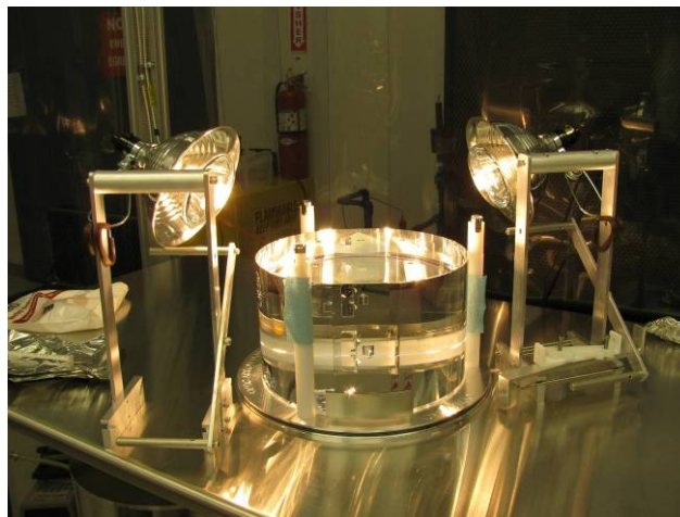
c) Two heat lamps on stands over PM ITM04 to help cure the adhesive
