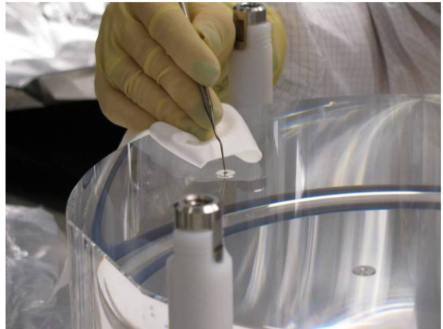
b) Close-up of gluing in a steel ring onto a mount disc using a pointy dental tool
