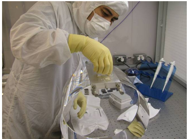
d) Placing the ear onto the bonding surface
