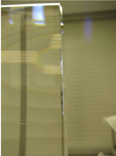
a) Scratches on the barrel at the chamfer
