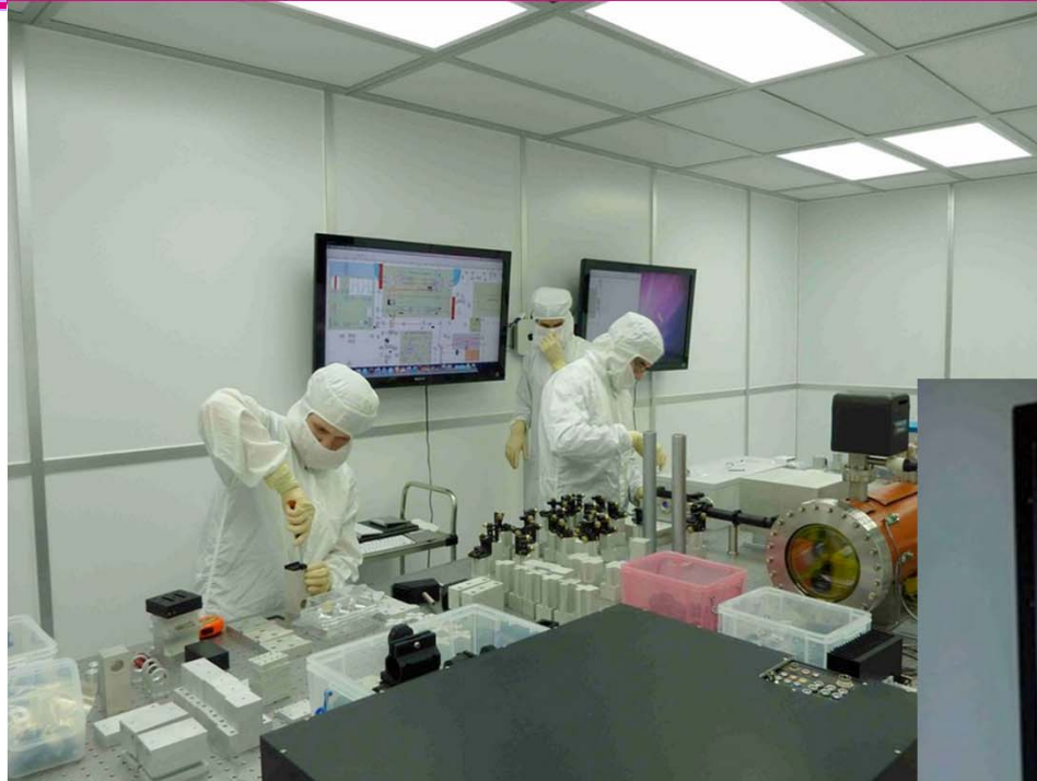
Laser Area Enclosure: HEPA filtered airflow & acoustic shielding
