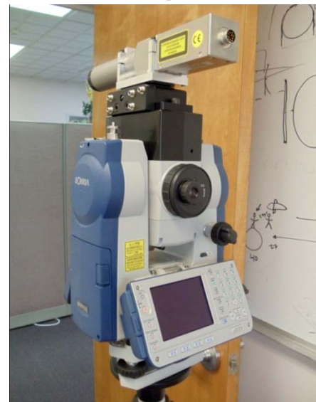
Laser Autocollimator co-boresighted with Total Station (theodolite)
