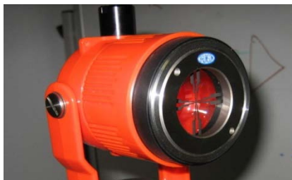
Cross-hair target integrated with retroreflector
