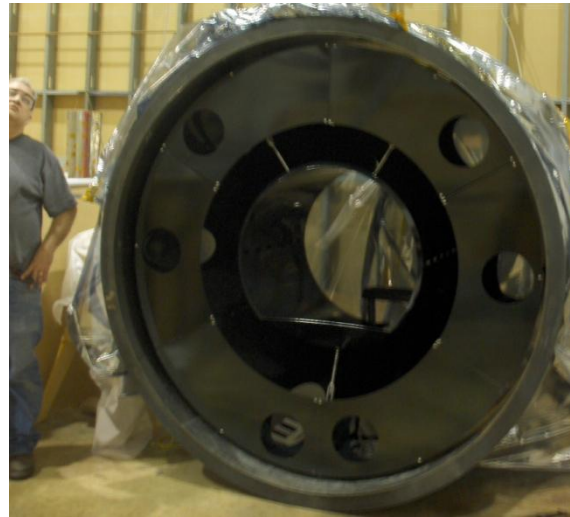
Manifold/Cryopump Baffle 1 st Article suspended inside manifold tube mock-up
