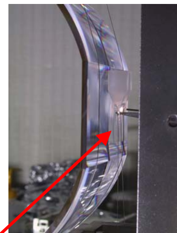
Silica fibres, length 600 mm diameter 400 \mu\text{m} , welded to silica ears
