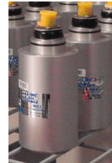
L4C f = \sim 1 Hz Inertial Sensor
