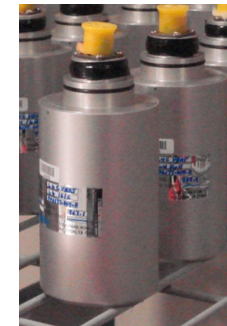
L4C f = \sim 1 Hz Inertial Sensor
