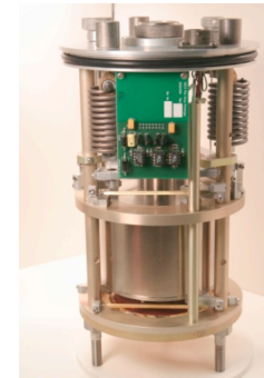
GS13 f = \sim 1 Hz Inertial Sensor
