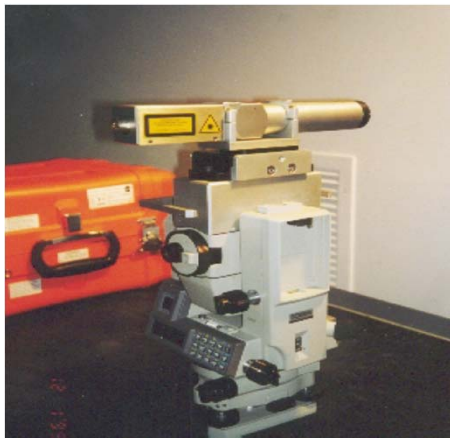
Photograph of the laser autocollimator mounted on the Sokkia Set2B for iLIGO.
