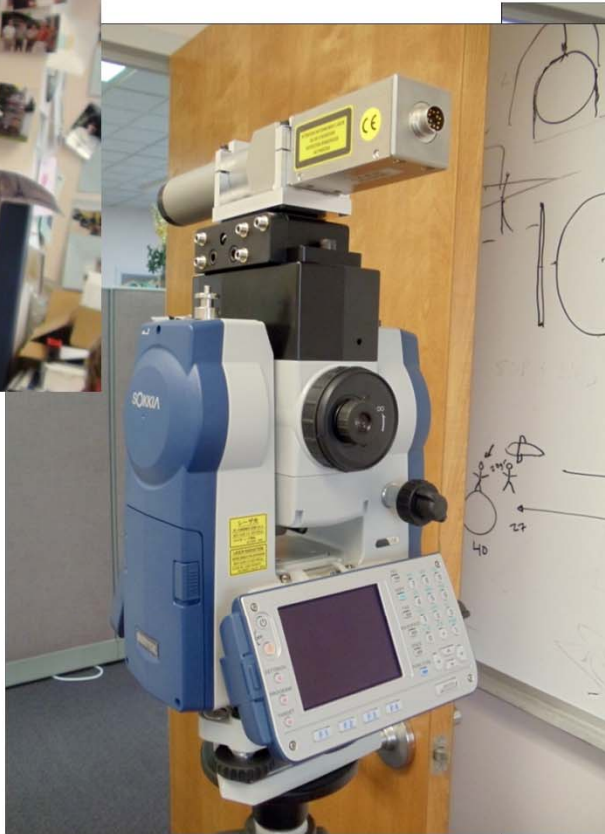
Sokkia model SetX1 with Newport Laser autocollimator mounted up
