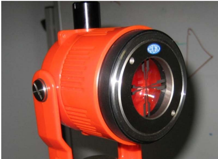
Above: Retro-reflectors with attached cross-hair target
