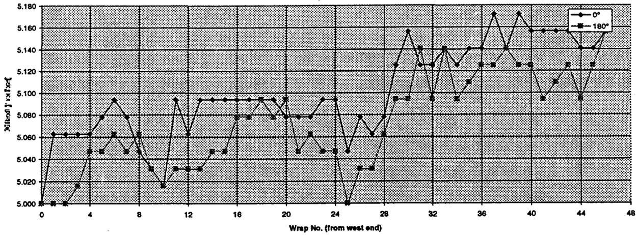
Diameter Measurements on 60' Beam Tube Section (21-3-2)
