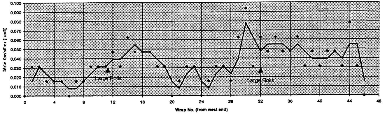
**Actual Standoff Measurements on 60' Beam Tube Section (21-3-2)**
