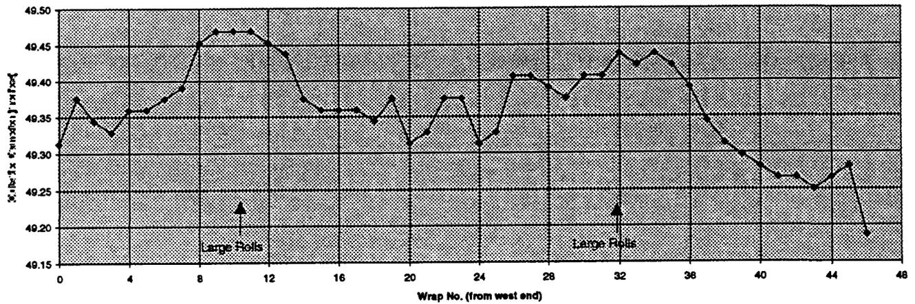
**Straightness Measurements on 60' Beam Tube Section (21-3-2)**
