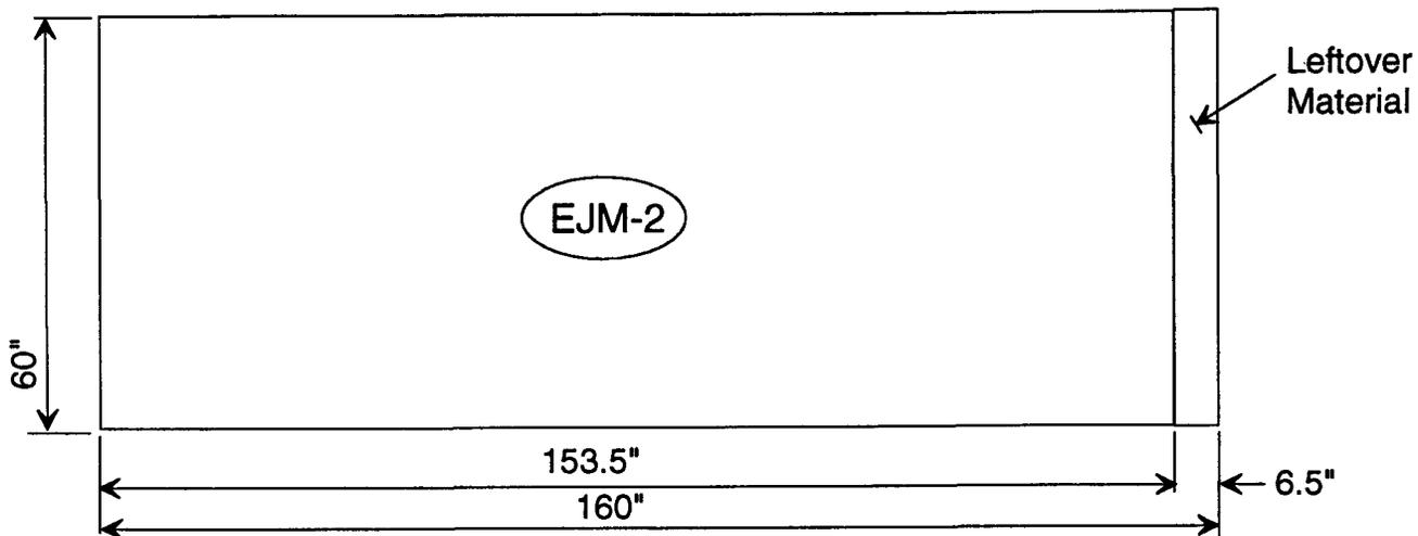
**HYSPAN EXPANSION JOINT MATERIAL (Three Required)**
