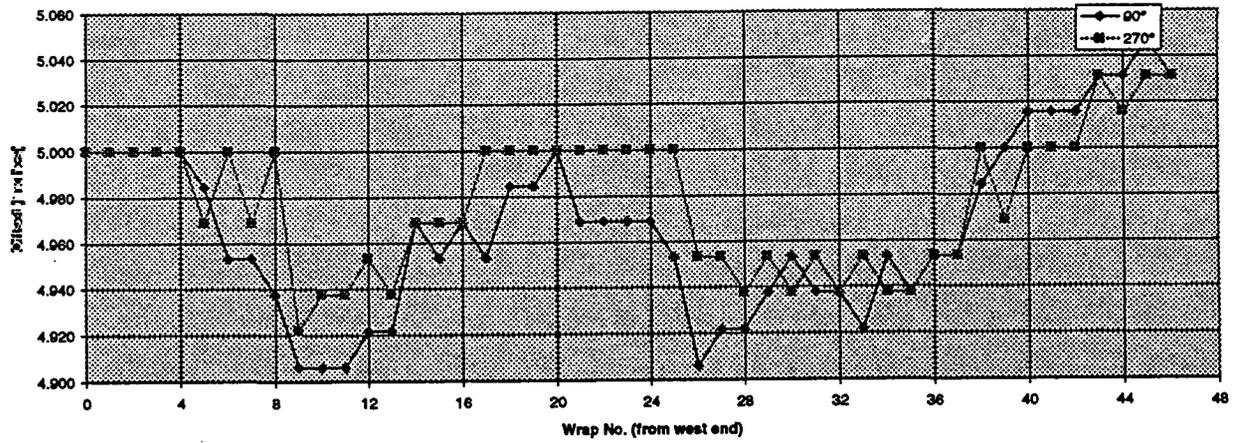
**Diameter Measurements on 60' Beam Tube Section (21-3-2)**
