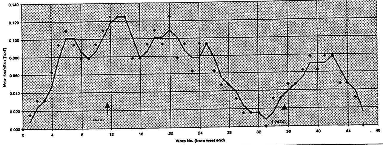
**Standoff Measurements on 60' Beam Tube Section (21-3-1)**
