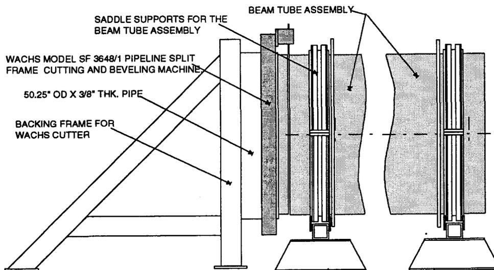
MACHINE SET UP TO CUT ENDS OF QT BEAM TUBE ASSEMBLIES
