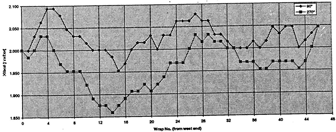
**Diameter Measurements on 60' Beam Tube Section (21-3-1)**
