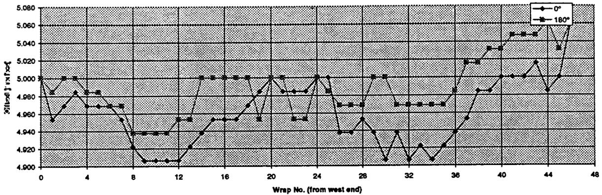
**Diameter Measurements on 60' Beam Tube Section (21-3-2)**
