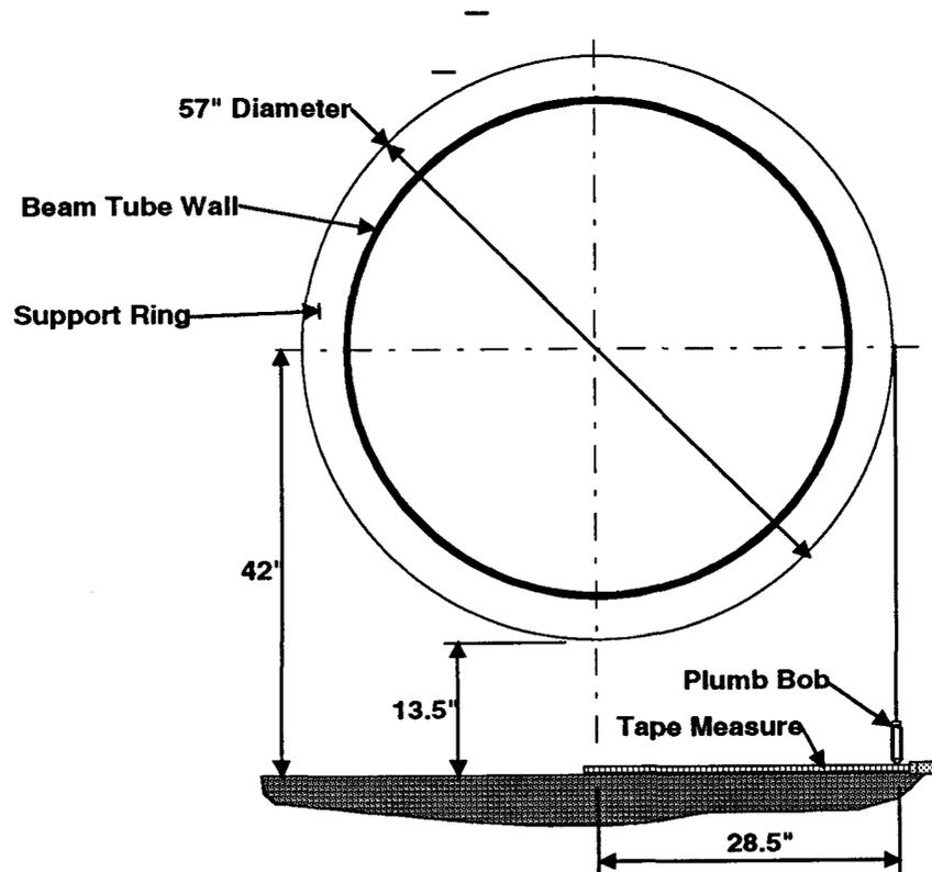
Next the 22B beam tube assembly was moved into position. The end of the 22B assembly (the expansion joint) was aligned and fit to the end of the 22A beam tube assembly. The guided support ring on the 22B assembly was rotated so that the holes in the support ring were clocked to match the holes in the guided support ring on the 22A assembly.
