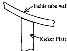
The gap was minimized and no melt through wall occurred.
