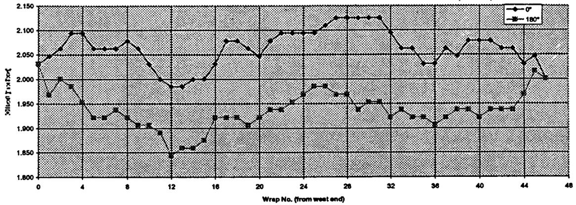
**Diameter Measurements on 60' Beam Tube Section (21-3-1)**
