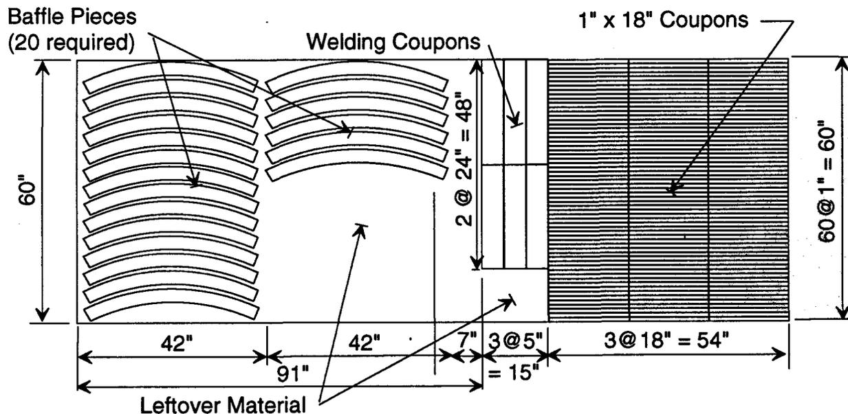
**MATERIAL FOR BAFFLES AND COUPONS (One Required)**
