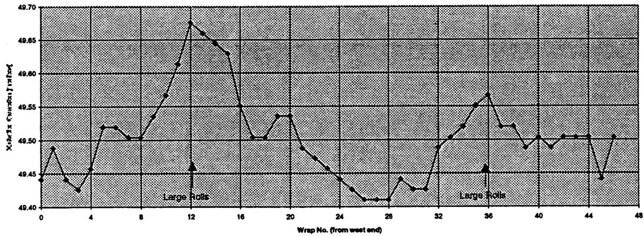
**Straightness Measurements on 60' Beam Tube Section (21-3-1)**
