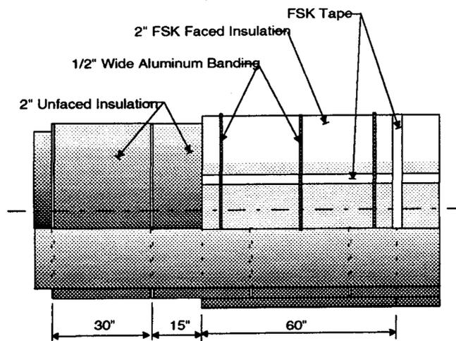
Insulation on QT Beam Tube Assembly
