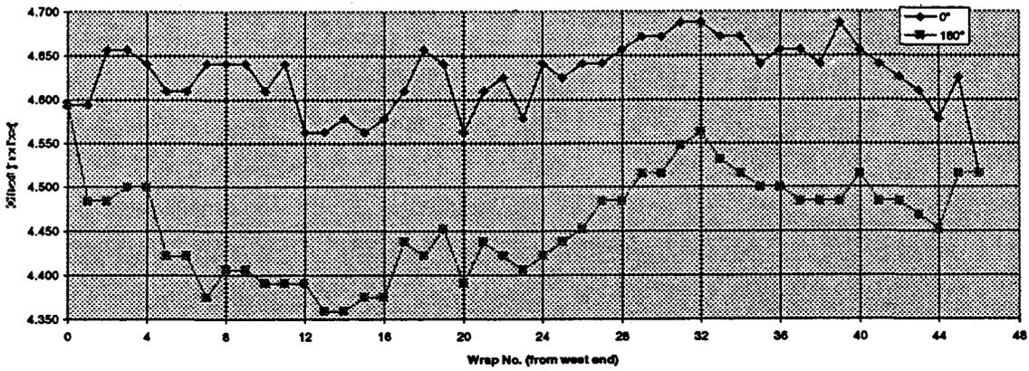
**Diameter Measurements on 60' Beam Tube Section (21-3-1)**
