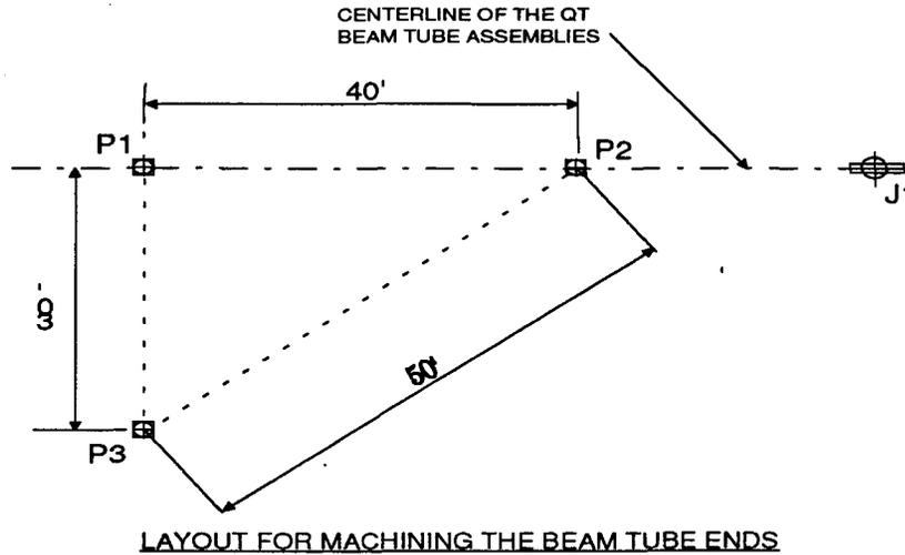
Next the pipe cut off machine was mounted onto the support frame. The frame was accurately plumbed and aligned to be perpendicular to the centerline of the beam tube using a jig transit in line with line P1-P3 and centered to the beam tube center line using a plumb bob. See the sketch below:
