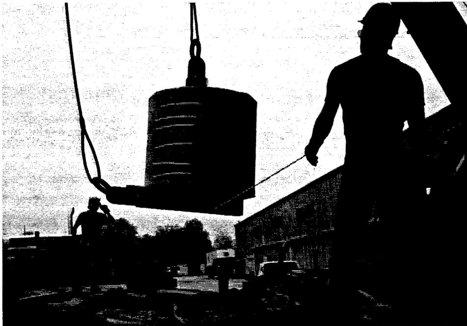
**Turning a Coil from Eye Horizontal to Eye Vertical for the Bake**
