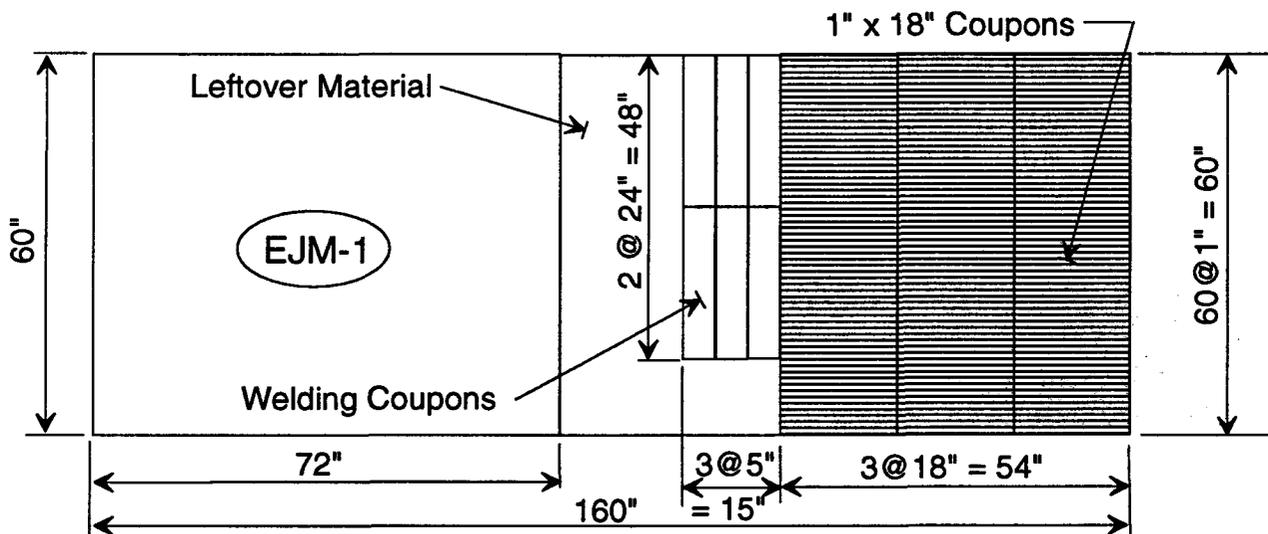
**MATERIAL FOR PATHWAY EXPANSION JOINT AND COUPONS (One Required)**
