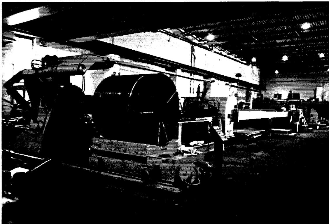
**Installing Coil into Stretcher Leveling Machine**
