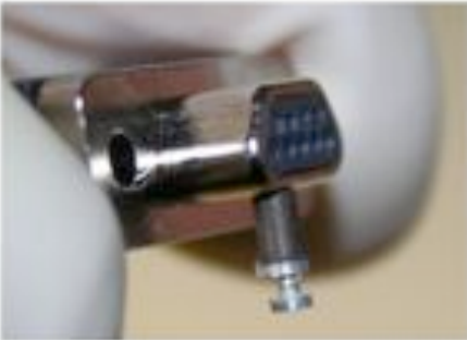
Connector (with suspended test mass magnet)
