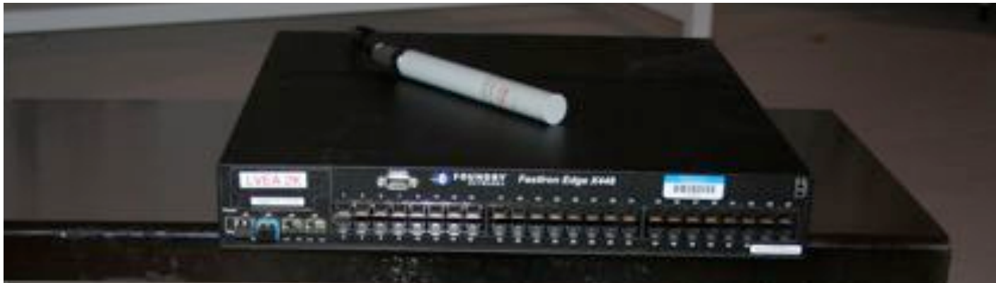
Magnetic field from Foundry X448, no connections other than AC power
