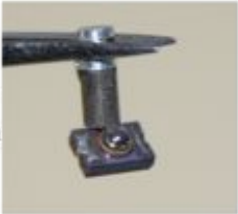
Diode chips, both transmitter and receiver, can be suspended from magnet
