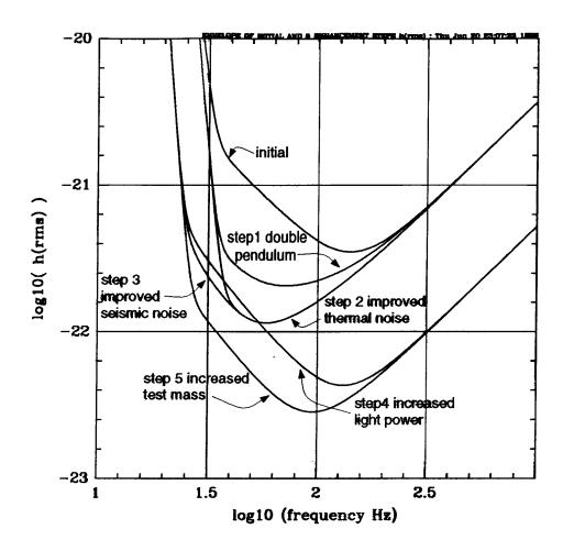
Figure 4: The improvements in  $h_{rms}$  associated with the steps outlined in the proposed program and resulting in the parameters given in Table 2. The logic of the steps is determined by the assumption that compact binary coalescences are the most likely source to be detected, hence the importance of improving the sensitivity near 100 Hz. The improvements associated with the do
