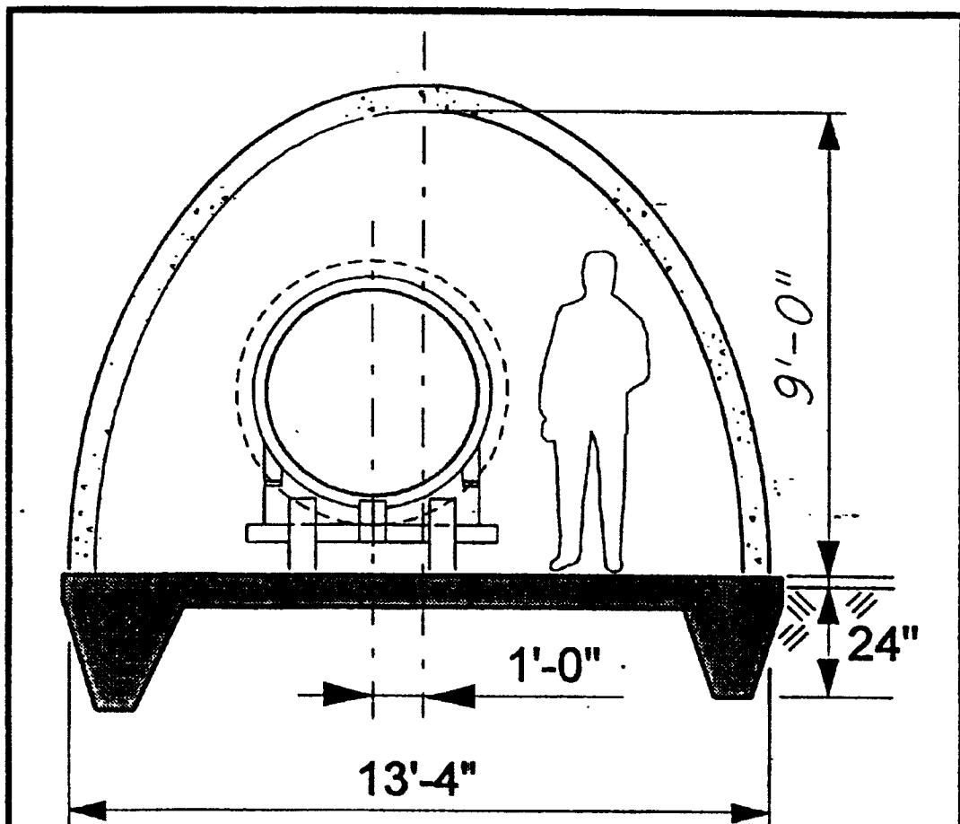
*Figure 2.1-1 – Cross Section of Design Baseline at Hanford*
