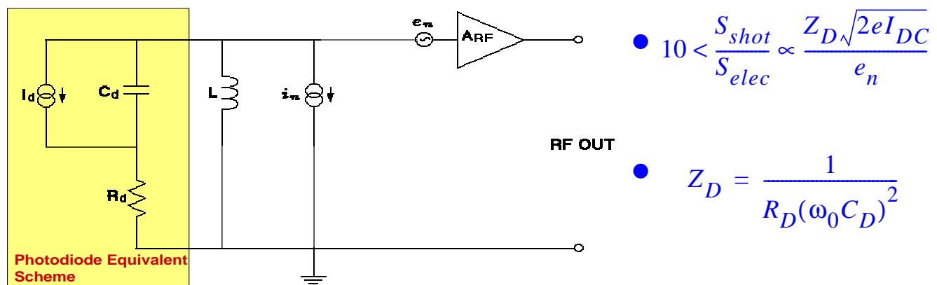
» need low diode resistance and capacitance
