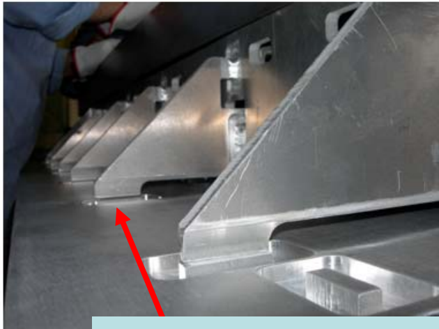
Weld shrinkage effect
