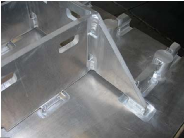
Weld shrinkage effect
