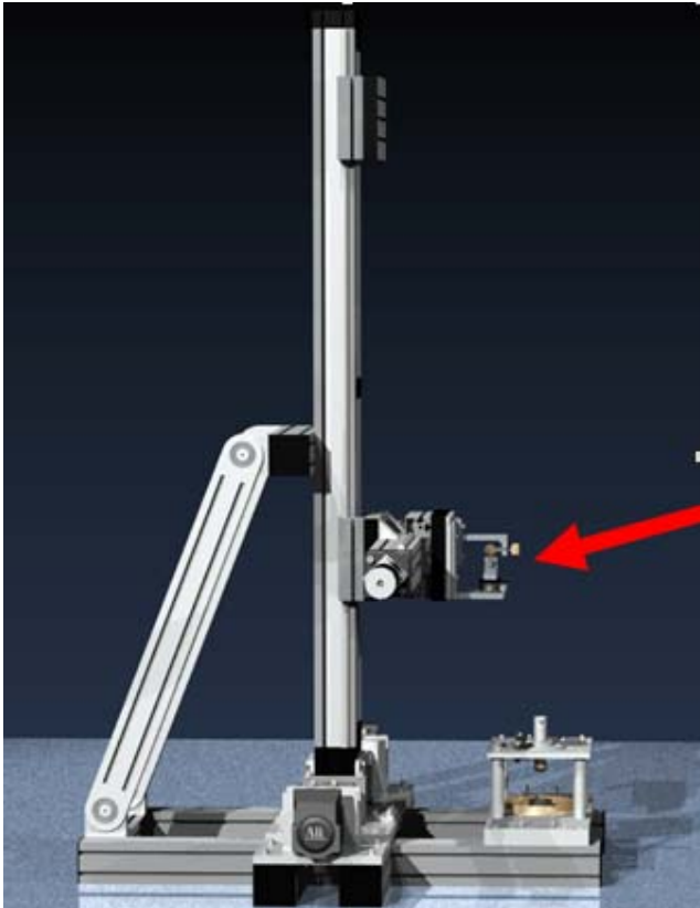
Glasgow CO 2 laser pulling & welding machine – welding configuration
