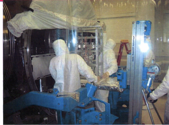
Mode Cleaner, Triple Suspension Installation in a HAM Chamber at LASTI
