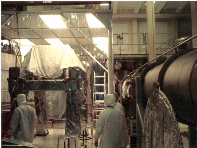
Quadruple Suspension Installation on Temporary Optics Table at LASTI
