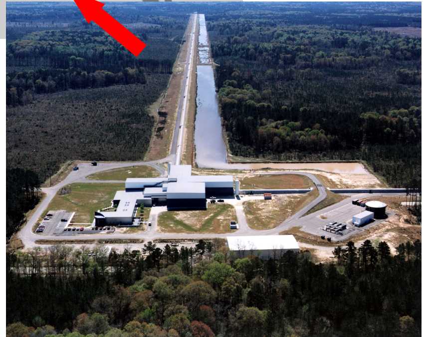
Livingston Observatory (L1) Single 4 km interferometer
