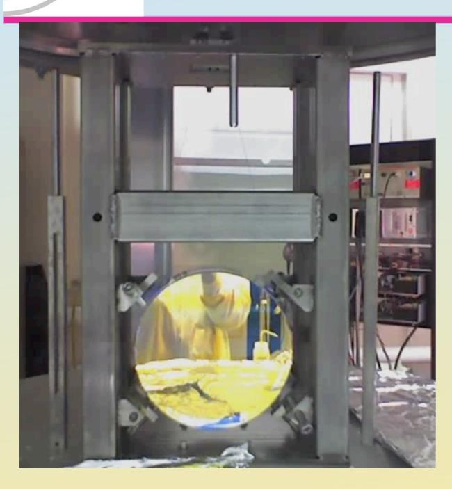
Pathfinder Optic hung in spare frame with wire from the sites. Each wire monitored by eight shadow sensors.
