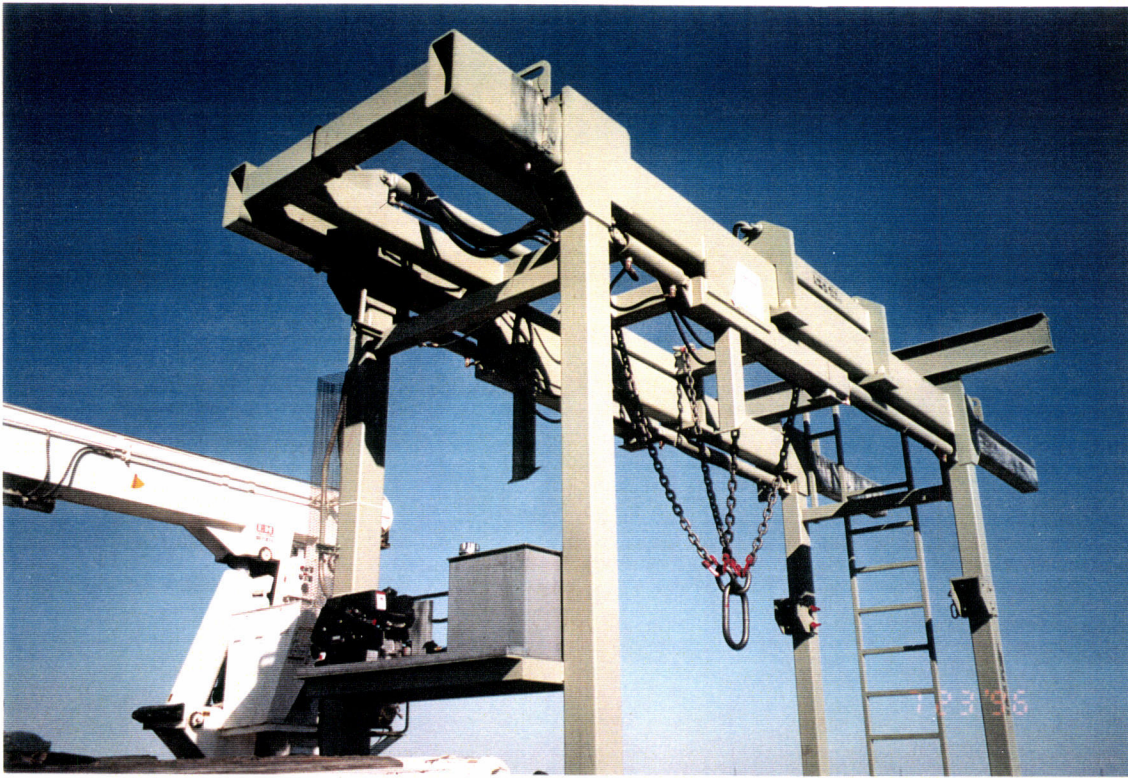
Closer view of the adjustable beams and rigging including the hydraulic pump and oil tank.
