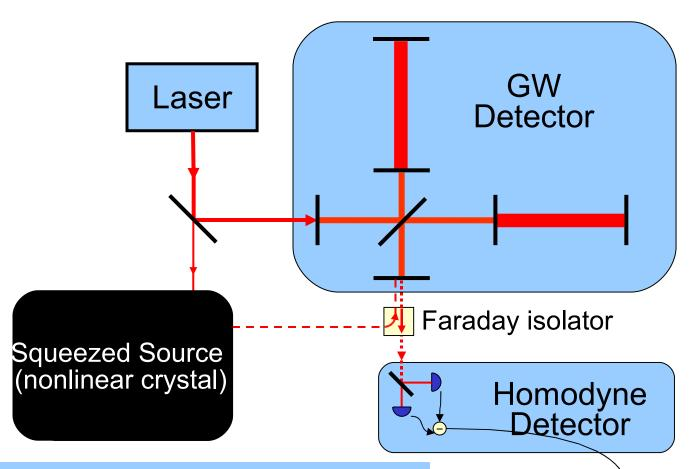
In principle, can reduce quantum noise by up to 10x at all frequencies.
