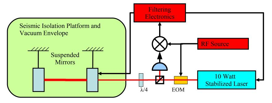
Detuned by inserting offset into PDH error signal, limited to detunings ~ half linewidth.
