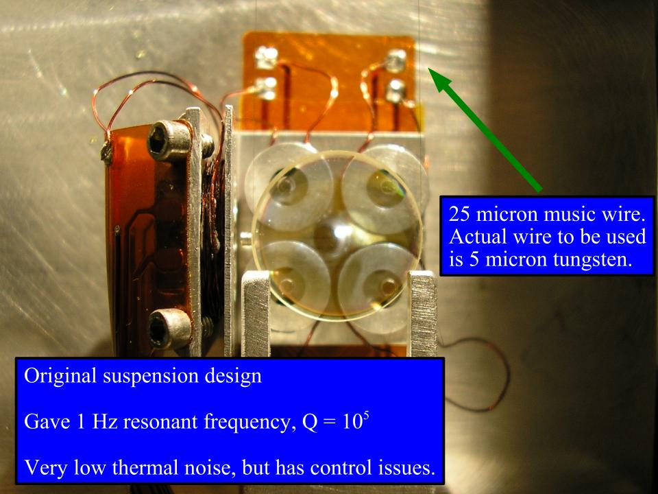
Easy suspension. Steel shell with same diameter as small optics. Suspended as a small optic with magnets, standoffs, etc. Little mirror attached by two 300 micron fused silica fibers. All glued together.
