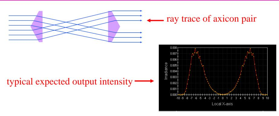
Axicons are lenses or mirrors with <u>conical</u> rather than <u>spherical</u> surfaces. They naturally convert incident centralized beams into output annular patterns.
