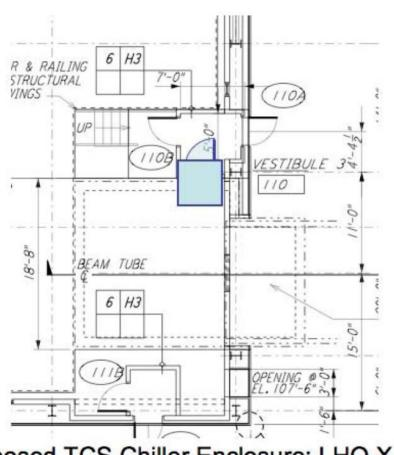
Chillers will be enclosed in closets far from the TCS table and optical lever piers- acoustic and electromagnetic interference should be minimized. Waste heat dumped into plenum air.
