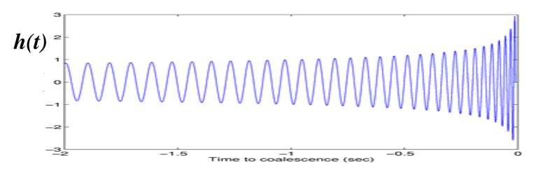
The "inspiral" will accelerate at the end, when the neutron stars coalesce Gravitational wave emission will be strongest near the end
