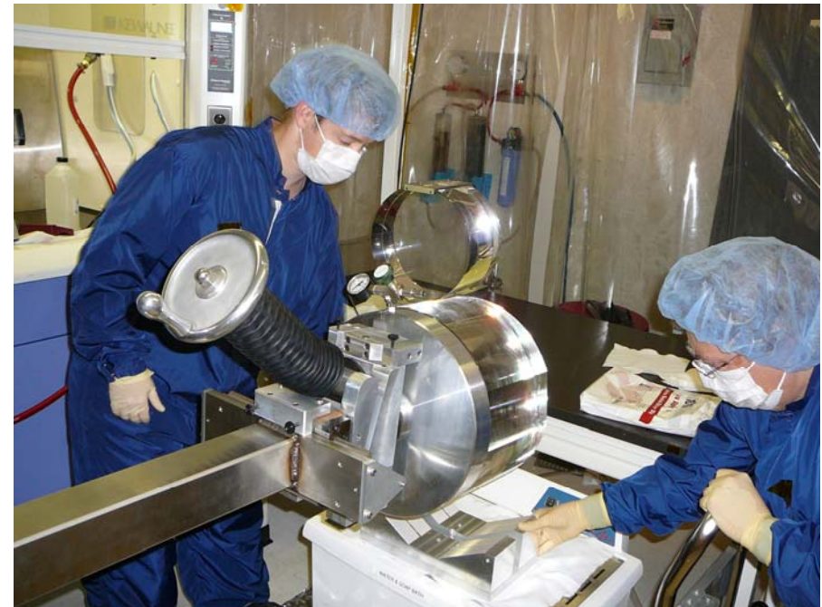
Step 4: Moving mass and lowering it on a V-block again
