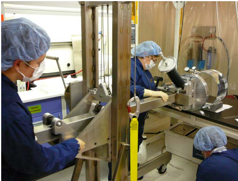
Step 1: Aligning the ergo-arm vacuum ring with the mass
