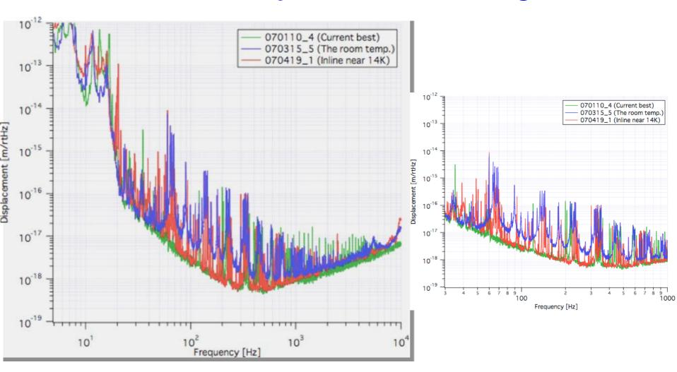
Inline near mirror was suspended by  $\Phi$ 1.0 Al wire. This is the first observation of sensitivity improvement by cooling.
