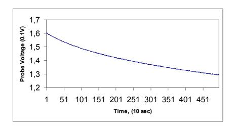
Time dependence of the peak height (fused silica sample with coating rotates, LED is switched on)
