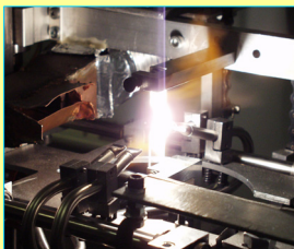
Pulling ribbon fibres using hydrogen-oxygen flame
