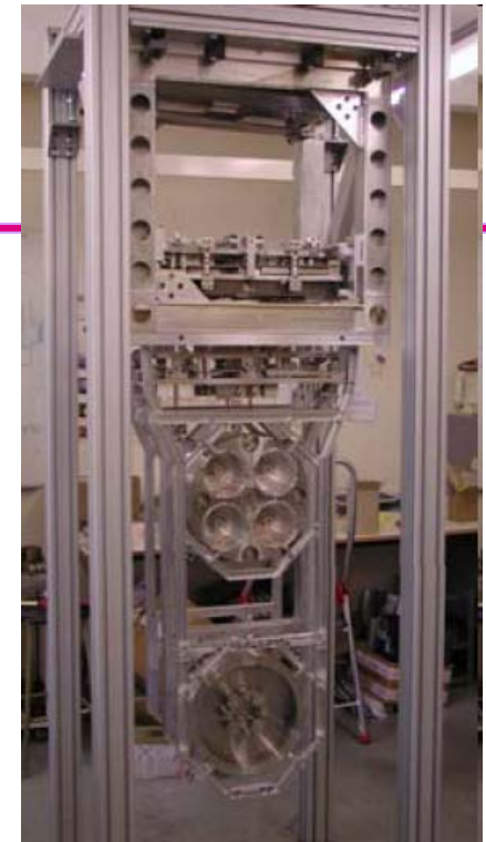
ETM/ITM Quadruple Pendulum Noise Prototype Assembly at RAL
