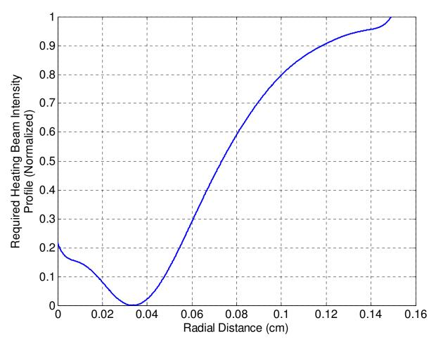
Heating beam pattern to be applied to a Fused Silica mirror to produce Mesa beam cavity mirrors
